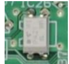
Polarity and existence of white photo couplers
