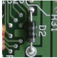
Polarity and existence of diodes
