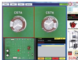
Inspection of a capacitor for wrong polarity - picture on right is the correct orientation
