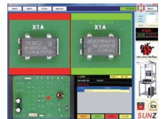
Inspection of an IC that was misplaced backwards and failed for polarity - picture on the right is the correct polarity
