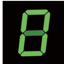
Brightness and lighting failure in each segment
