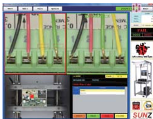
Inspection of wires in an final assembly process - picture on right is the correct wire arrangement
