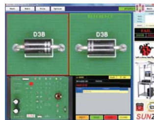
Inspection of a diode for wrong polarity - picture on the right is the correct polarity
