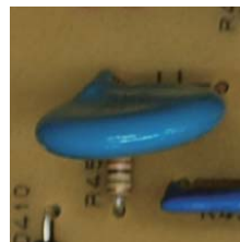
Excessive inclination of parts
