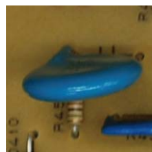
Excessive inclination of parts
