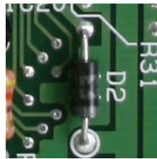
Polarity and existence of diodes
