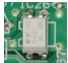
Polarity and existence of white photo couplers
