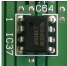
Polarity and existence, wrong pin number for IC
