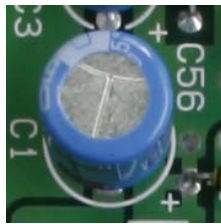
Polarity and existence of electrolytic capacitor
